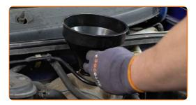
Pour coolant in the coolant reservoir.
