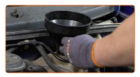
Pour coolant in the coolant reservoir.
