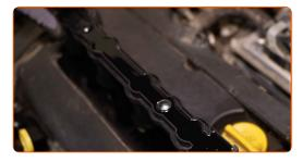
Tighten the ignition coil bolts. Use Torx T40. Use a torque wrench. Tighten it to 7 nm torque.
