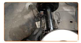
Tighten the stabiliser link fastener. Use a combination spanner #18.
