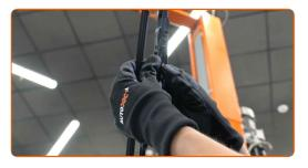
Remove the blade from the wiper arm.
