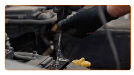
Treat the ignition coil connector with electronic spray. The spray will protect the electrical contacts from corrosion, oxidation, and will reduce the contact resistance.
