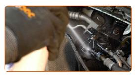
Unscrew the fasteners of the fuel filter housing cover. Use Torx T30. Use a ratchet wrench.
