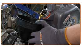
Replacement: engine oil and filter – OPEL Frontera A Off-Road (U92). AUTODOC experts recommend:
