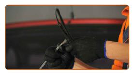
Remove the blade from the wiper arm.
