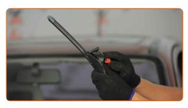
A Remove the blade from the wiper arm.
