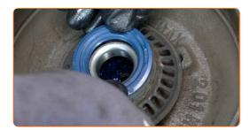
Treat the stub axle. Use all-purpose cleaning spray. Use bearing grease.
