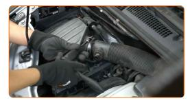
Treat the mass air flow sensor connector. Use electronic spray.
