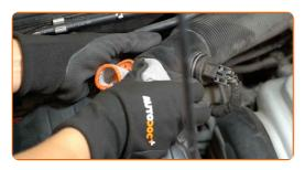
6 Unplug the mass air flow sensor connector.
