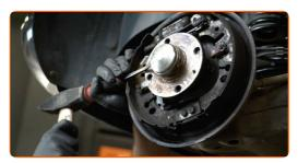
Replacement: wheel bearing – OPEL Corsa C Van (X01). AUTODOC experts recommend:
