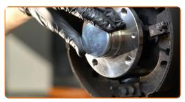
Treat the wheel hub in the area where it contacts the brake drum. Use copper grease.
