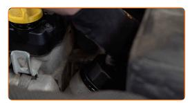
Screw the cap. Use a drive socket #32. Use a torque wrench. Tighten it to 15 Nm torque.
