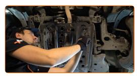
Remove the oil pan cover. Use a drive socket #12. Use a ratchet wrench.
