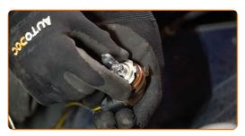
Replacement: headlight bulb – OPEL Corsa C Van (X01). AUTODOC recommends:
