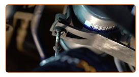
Remove the fuel filter. Put the old filter cartridge in the container.
