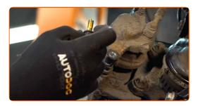
10 Remove the brake caliper.
