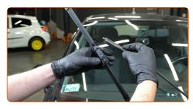
Replacement: windshield wipers – OPEL Corsa E Hatchback (X15). Professionals recommend:
