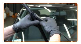
Remove the blade from the wiper arm.
