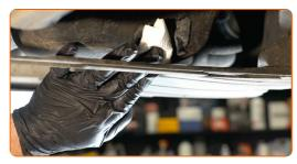
Screw in the new drainage plug and tighten it. Use Torx T45. Use a torque wrench. Tighten it to 20 Nm torque.
