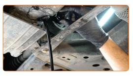
Replacement: engine oil and filter – OPEL Corsa E Hatchback (X15). Tip:
