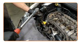
Install the protective case of the oil filter housing.
