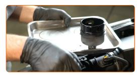
Replacement: engine oil and filter – OPEL Corsa E Hatchback (X15).
