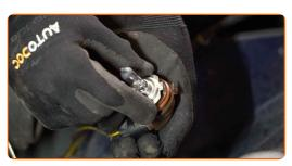
Replacement: headlight bulb – OPEL Corsa D Hatchback (S07). AUTODOC recommends:
