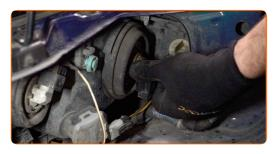
Remove the old bulb. Use a flat screwdriver.
