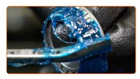
21 Install a new hub bearing and secure it.
