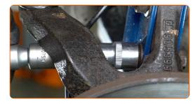
Treat the shock strut fasteners. Treat the fastener connecting the tie rod end to the steering knuckle. Treat the CV axle fastener. Treat the fasteners of the ball joint. Use copper grease.
