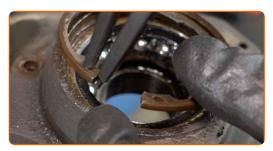
Press out the wheel hub bearing. Use a bush and bearing driver set.
