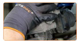
Tighten the brake caliper bracket. Use HEX No.H10. Use a torque wrench. Tighten it to 95 Nm torque.
