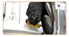
Tighten the oil filler cap.
