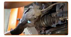
Tighten the brake caliper bracket. Use a drive socket #E20. Use a torque wrench. Tighten it to 100 Nm torque.
