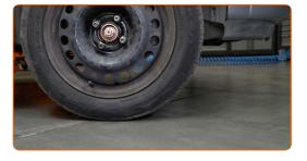
Tighten the drive shaft nut. Use a drive socket #30. Use a torque wrench. Tighten it to 177 Nm torque.
