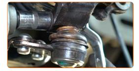
Tighten the ball joint fastener. Use a combination spanner #16. Use a drive socket #16. Use a torque wrench. Tighten it to 55 Nm torque.
