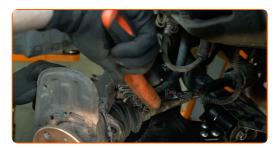
Unscrew the fasteners connecting the suspension strut to the steering knuckle. Use a combination spanner #18. Use a drive socket #18. Use a tap wrench.
