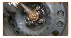
Tighten the wheel bolts using a criss-cross pattern. Use a torque wrench. Tighten it to 110 Nm torque.
