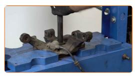
Clean the fasteners of the wheel hub bearing. Use a wire brush. Use WD-40 spray.
