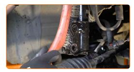
Install the steering knuckle assembled with the wheel hub.
