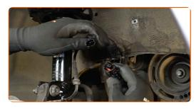
Disconnect the ABS sensor wiring.
