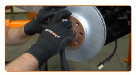
Remove the brake disc.
