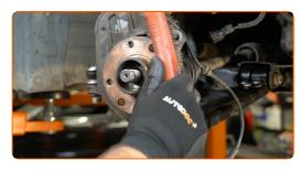
64 Install the brake disc.
