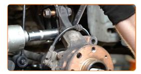
Tighten the lower fasteners connecting the shock strut to the steering knuckle. Use a combination spanner #18. Use a drive socket #18. Use a torque wrench. Tighten it to 80 Nm torque.+60°
