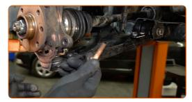
Disconnect the lower arm from the steering knuckle.
