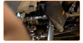
Attach the ABS sensor connector.
