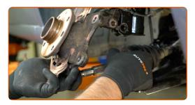
Remove the fastening bolt.
