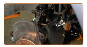
Unscrew the fastener connecting the ball joint to the steering knuckle. Use a combination spanner #16. Use a drive socket #16. Use a ratchet wrench.
