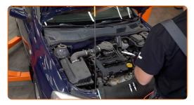
Screw new spark plugs and tighten them. Use the spark plug socket #16. Use a torque wrench. Tighten it to 24 nm torque.
