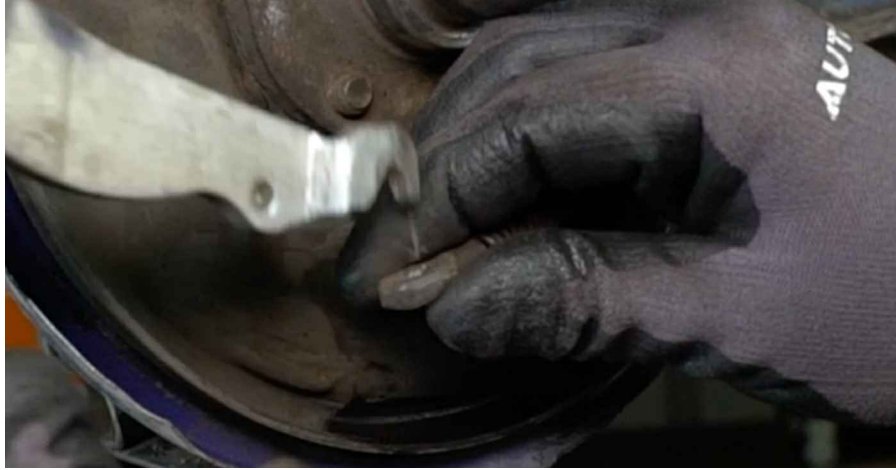
21 Remove the left brake shoe.
