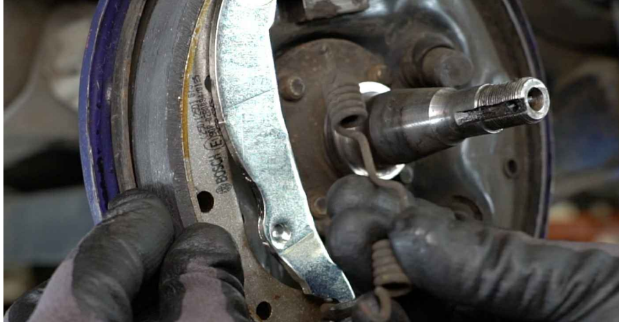
25 Install the lower return spring.
