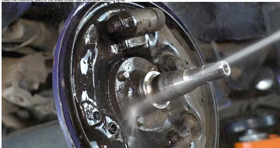
Replacement: brake shoes – OPEL Corsa C Van (X01). Tip from AUTODOC experts:
