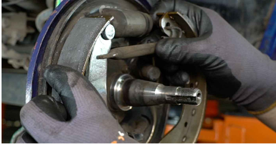
37 Install the lower return spring.
