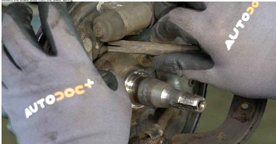
18 Remove the right brake shoe.
