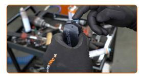
Replacement: brake pads – OPEL Corsa C Van (X01). Tip from AUTODOC:
