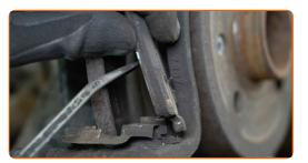
Replacement: brake pads – OPEL Corsa C Van (X01). Tip from AUTODOC experts:
