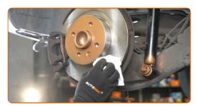
Replacement: brake pads – OPEL Corsa C Van (X01). Professionals recommend:
