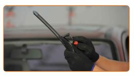
Remove the blade from the wiper arm.
