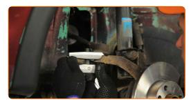
Loosen the lock nut securing the tie rod end to the tie rod. Use a combination spanner #19.
