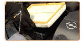
Cover the air intake hose with a microfibre towel to prevent dust and dirt from getting into the system.
