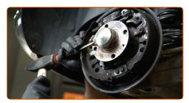
Replacement: wheel bearing – OPEL Corsa C Hatchback (X01). AUTODOC experts recommend:
