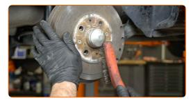
Unscrew the brake drum fastening Use Torx T30. Use a ratchet wrench.
