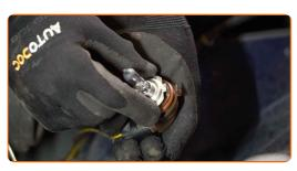
Replacement: headlight bulb – OPEL Corsa C Hatchback (X01). AUTODOC recommends:
