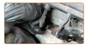
Unscrew the glow plugs. Use the spark plug socket #8. Use a ratchet wrench.
