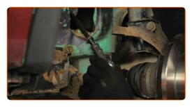
Replacement: track rod end – OPEL Corsa B Van (S93). Professionals recommend:
