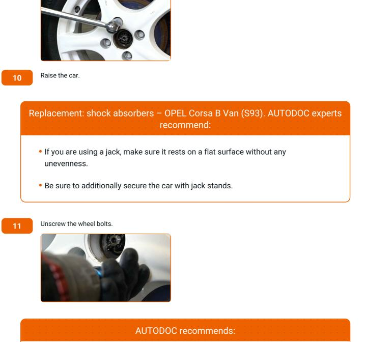
Loosen the wheel mounting bolts. Use wheel impact socket #17.
