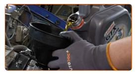
Replacement: engine oil and filter – OPEL Corsa B Van (S93). AUTODOC experts recommend:
