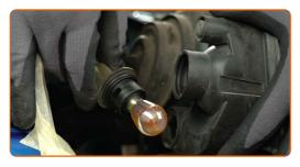
Install the bulb holder together with the bulbs.
