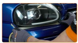
3 Unscrew the headlight fasteners. Use a Phillips screwdriver.
