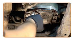
10 Remove the transmission fluid pan.
