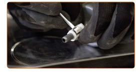
Install the retainers of the fasteners of the fuel filter tubes.
