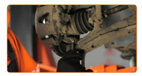
Remove the fastening bolt. Use a hammer.
