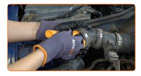
6 Release the air filter cover clips.
