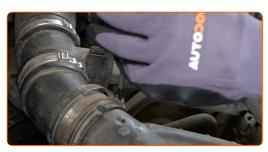
Disconnect the air intake pipe from the air filter housing.
