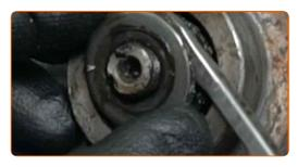
Remove the wheel hub bearing. Use a crowbar.
