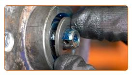
Screw on the hub nut. Use a drive socket #24. Use a ratchet wrench.
