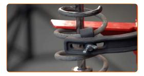
Remove the assembled shock strut.
