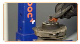
Remove the strut piston rod nut. Use a flat screwdriver. Use a drive socket #19. Use a ratchet wrench.
