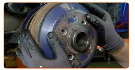
Replacement: wheel bearing - OPEL Corsa A Van (S83). Tip from AUTODOC:
