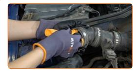
6 Release the air filter cover clips.
