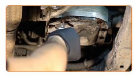
10 Remove the transmission fluid pan.
