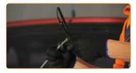
Remove the blade from the wiper arm.
