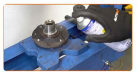
Pull the bearing inner race out of the wheel hub. Use a bearing separator. Use a bush and bearing driver set.
