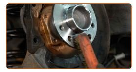
23 Install the brake disc.
