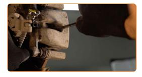
Remove the brake caliper. Use a crowbar.
