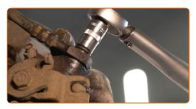
Remove the brake hose clamp.
