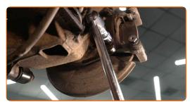
18 Remove the caliper bracket.
