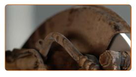
Clean dirt from the brake hose bolt. Use a wire brush. Use a brake cleaner.
