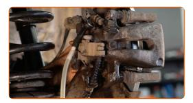
Bleed the brake caliper system. Without starting the engine, press the brake pedal several times until you feel significant resistance.
