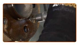
Remove the brake disc.
