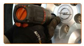
Lower the car and working in a cross order, tighten the wheel bolts. Use a torque wrench. Tighten it to 110 Nm torque.
