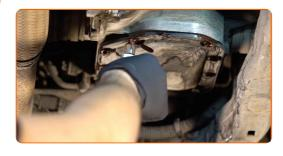
10 Remove the transmission fluid pan.
