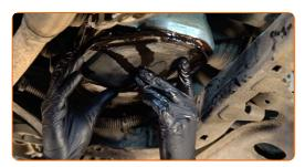
Replacement: manual gearbox oil – OPEL Combo Platform / Chassis (X12). Tip:
